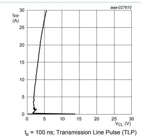
Fig. 7. Dynamic resistance with positive clamping voltage
