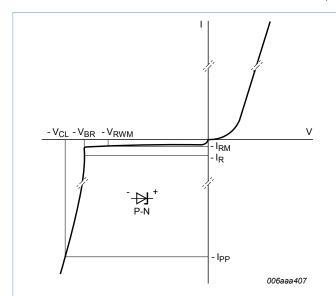
Fig. 3. V-I characteristics for unidirectional ESD protection diode
