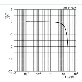
Fig. 6. Insertion loss; typical values
