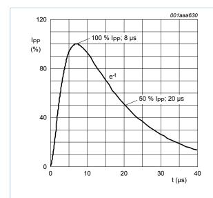
Fig. 1. 8/20 µs pulse waveform according to IEC 61000-4-5 and IEC 61643-321
