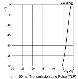
Fig. 8. Dynamic resistance with negative clamping
