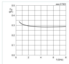
Fig. 5. Diode capacitance as a function of frequency; typical values
