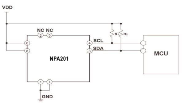
Figure 7 - Hardware pin connection diagram
