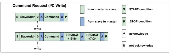
Figure 3 - I<sup>2</sup>C Command Request
