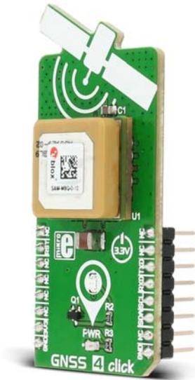
**GNSS 4 click** carries SAM-M8Q patch antenna module from u-blox. The click is designed to run on a 3.3V power supply. It communicates with the target microcontroller over I2C or UART interface.
