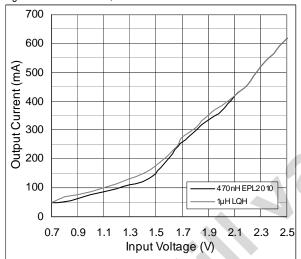
Figure 11. Powersave Threshold vs. VIN
