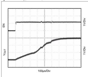
Figure 16. Shutdown, VOUT = 3V, IOUT = 1mA
