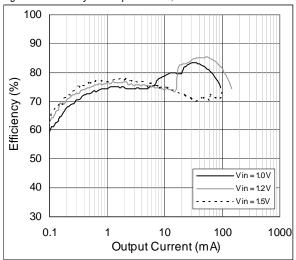
Figure 5. Efficiency vs. Output Current, Vout = 3.0V
