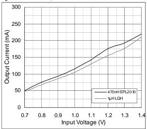
Figure 10. IOUT vs. VIN; VOUT = 3.0V
