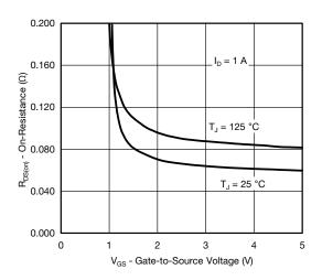
On-Resistance vs. Gate-to-Source Voltage
