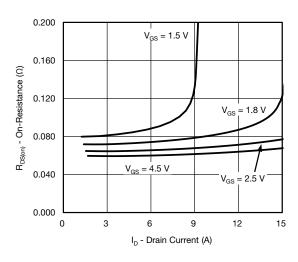
On-Resistance vs. Drain Current
