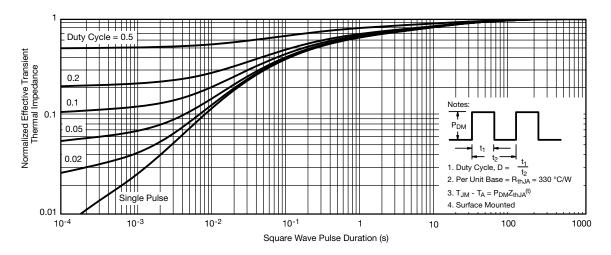
Normalized Thermal Transient Impedance, Junction-to-Ambient (on 1" x 1" FR4 board with minimum copper)
