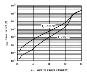
Gate Current vs. Gate-Source Voltage
