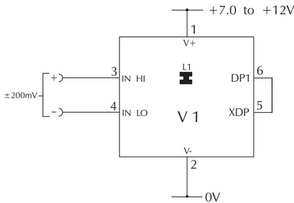
Measuring an input voltage referenced to a floating supply, i.e. the input voltage and the meter's power supply are isolated from each other. Check Link L1 is closed.
