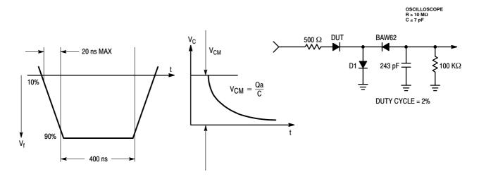
Figure 2. Stored Charge Equivalent Test Circuit
