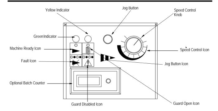
The green indicator on the top of the control panel indicates the machine status.
