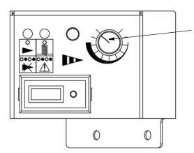
When the Dial is Turned Fully Counterclockwise, the Indicator on the Dial Should Align with the Indicator on the Control Panel
