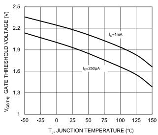
Figure 8. Gate Threshold Variation vs Temperature
