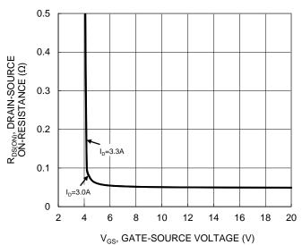
Figure 4. Typical Transfer Characteristic
