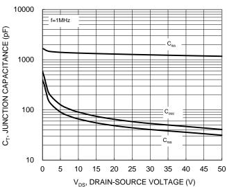
$V_{\rm DS}$ , DRAIN-SOURCE VOLTAGE (V) Figure 10. Typical Junction Capacitance
