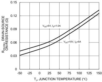
Figure 7. On-Resistance Variation with Temperature
