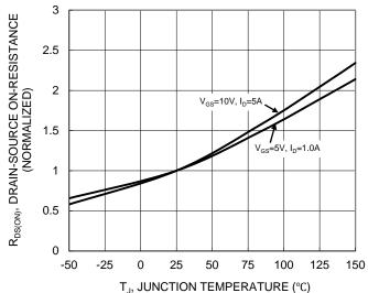
Figure 6. On-Resistance Variation with Temperature
