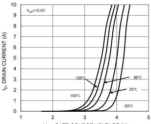
$V_{\rm GS}$ , GATE-SOURCE VOLTAGE (V) Figure 2. Typical Transfer Characteristic
