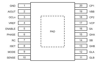
Package ES, 20-Pin QFN Pin-Outs
