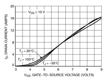
Figure 2. Transfer Characteristics
