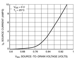
Figure 10. Diode Forward Voltage versus Current
