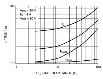
Figure 9. Resistive Switching Time Variation versus Gate Resistance
