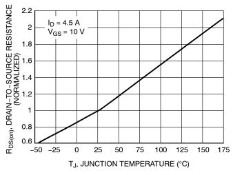
Figure 5. On–Resistance Variation with Temperature
