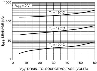
Figure 6. Drain-To-Source Leakage Current versus Voltage
