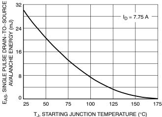
Figure 12. Maximum Avalanche Energy versus Starting Junction Temperature
