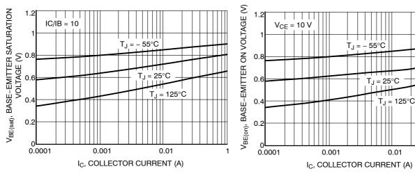
Figure 3. Base Saturation Voltage
