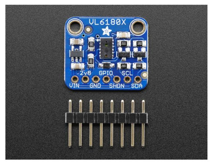
The sensor is small and easy to use in any robotics or interactive project. Since it needs 2.8V power and logic we put the little fellow on a breakout board with a regulator and level shifting. You can use it with any 3-5V power or logic microcontroller with no worries. Each order comes with a small piece of header. Solder the header onto your breakout board with your iron and some solder and wire it up for instant distance-sensing-success!
