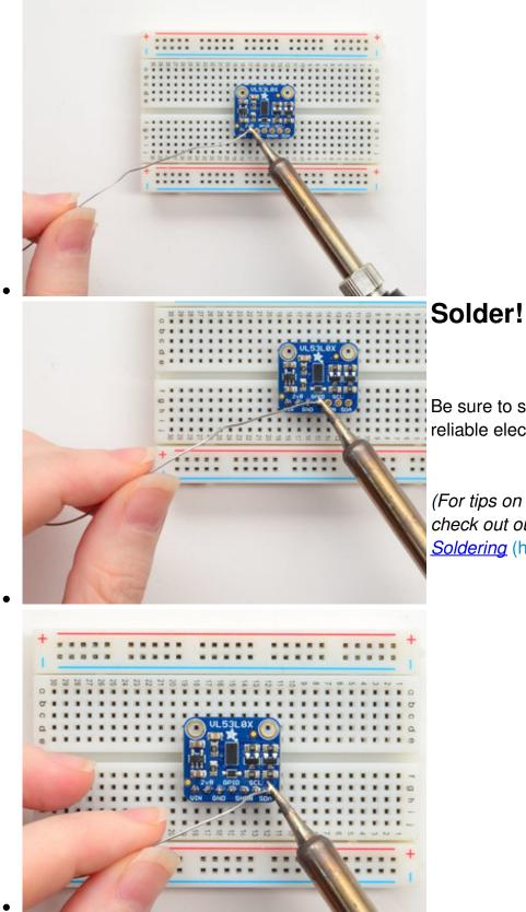
Be sure to solder all pins for reliable electrical contact.
