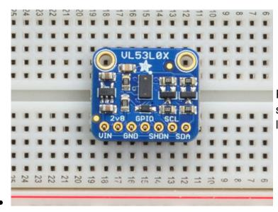
Place the Breakout board on top so the shorter ends of the pins line up though all the pads
