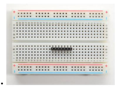
Cut the strip to length if necessary. It will be easier to solder if you insert it into a breadboard - **long pins down**
