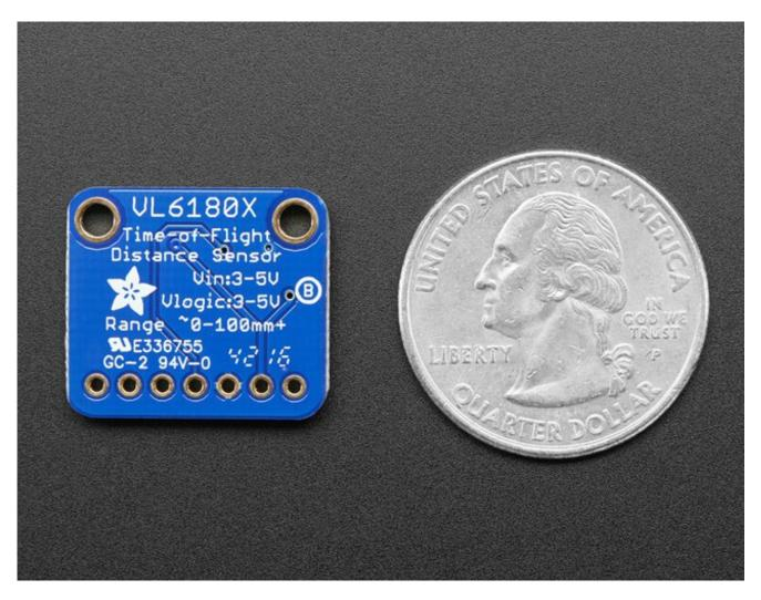
Communicating to the sensor is done over I2C with some simple commands. Most of the work is handled inside the sensor itself, so its very easy to port our Arduino library to another microcontroller.
