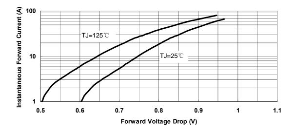
Fig.3-Typical Instantaneous Forward Voltage Characteristics
